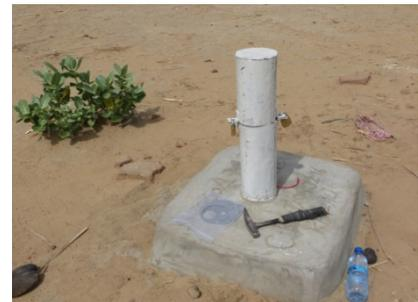
A data logger hanging inside the borehole by means of a ring. Installation of a data logger inside the borehole
