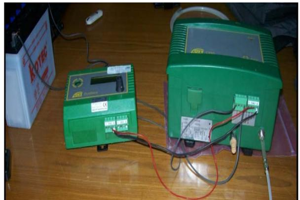
DuoSens recorder for hydrometry
